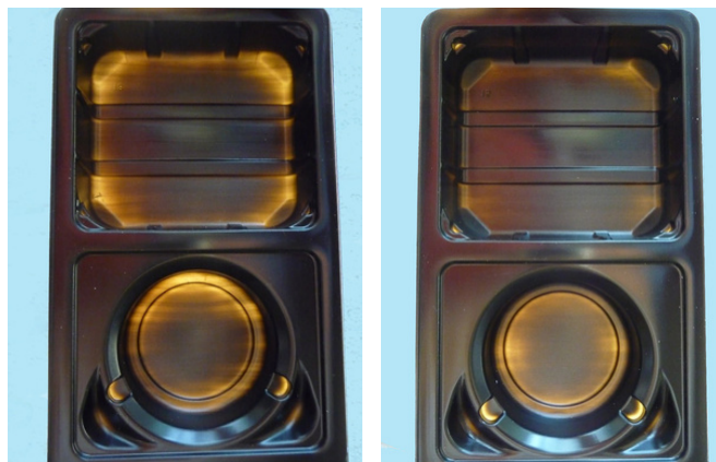
Control - No MPM 2000 1% MPM 2000 MPM 2000 = More uniform wall thickness thereby eliminating thin spots at the tray corners
